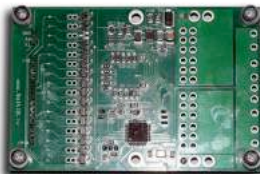
Battery Management System
